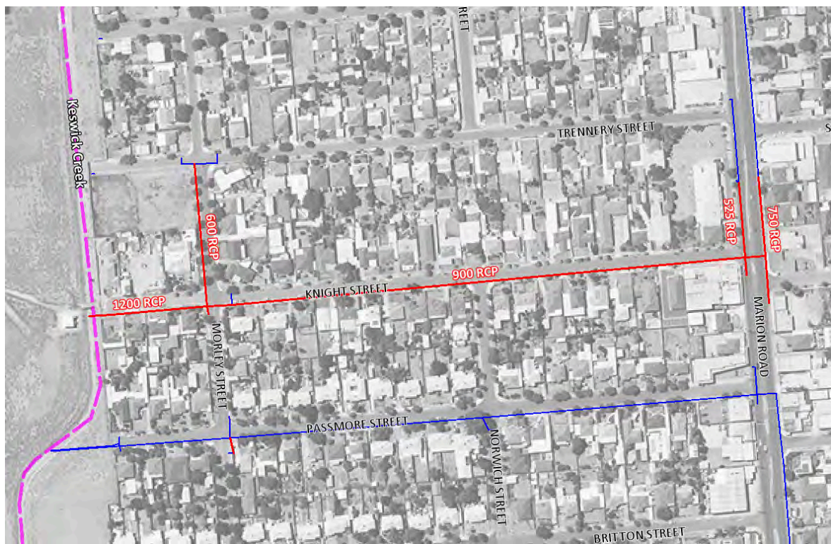
Figure 4.59 – Knight Street Drainage Layout
