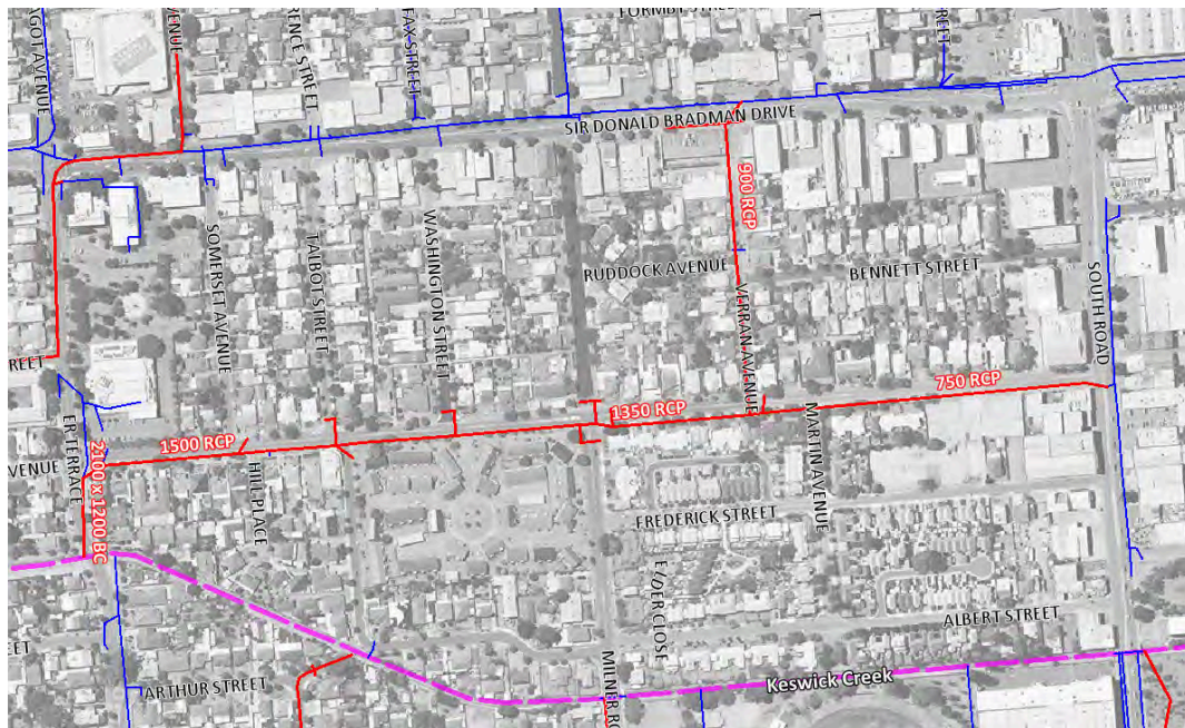
Figure 4.51 – Davenport Terrace Drainage Layout
