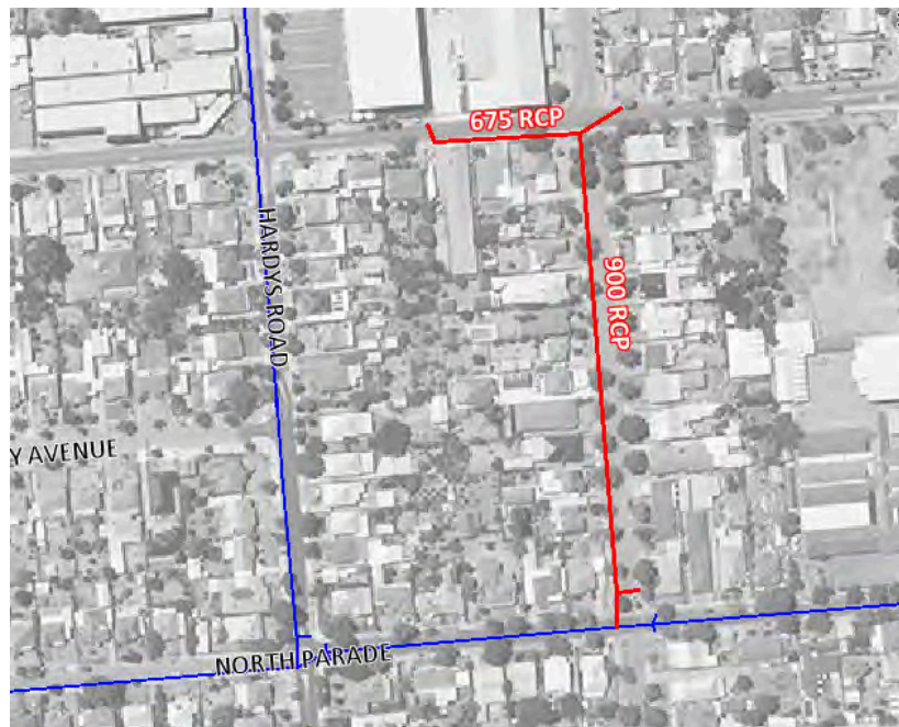
Figure 4.42 – Stephens Avenue Drainage Layout
