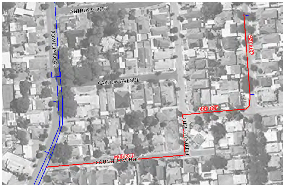
Figure 4.34 – Malurus Avenue Drainage Layout
