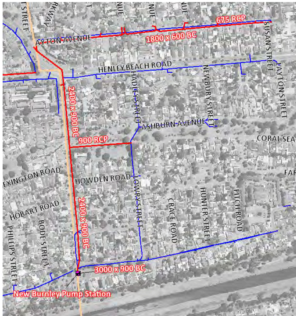
Figure 4.27 – Burnley Street Pump Station and Drainage Layout
