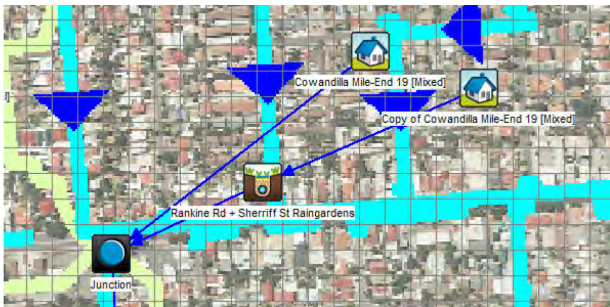
Figure 5.3 – Example of MUSIC subcatchment being separated by ‘area being treated by raingardens’ and ‘area with no treatment’
