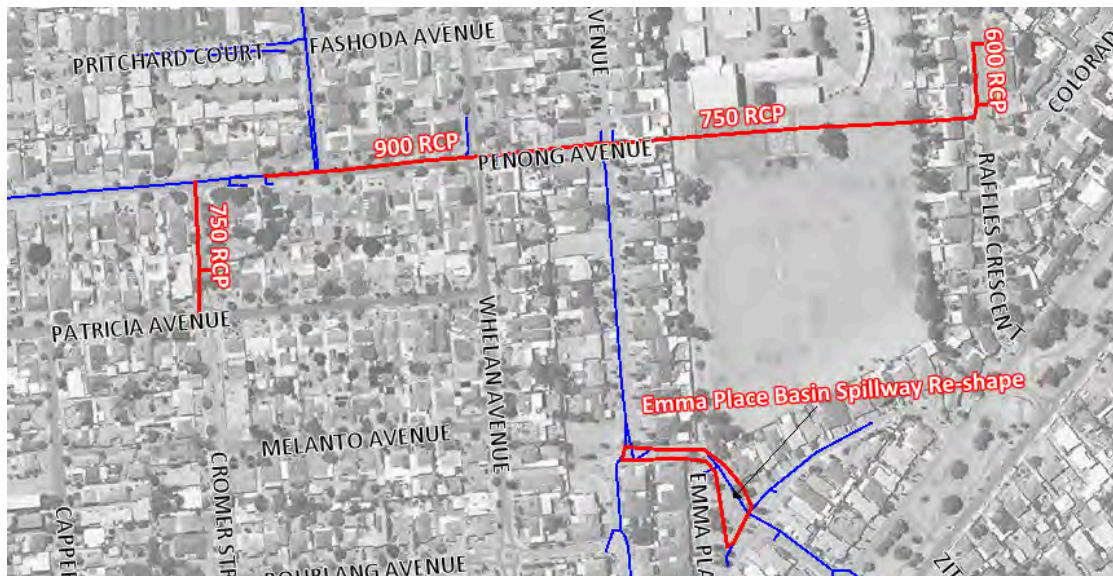
Figure 4.74 – Penong Avenue Drainage Layout
