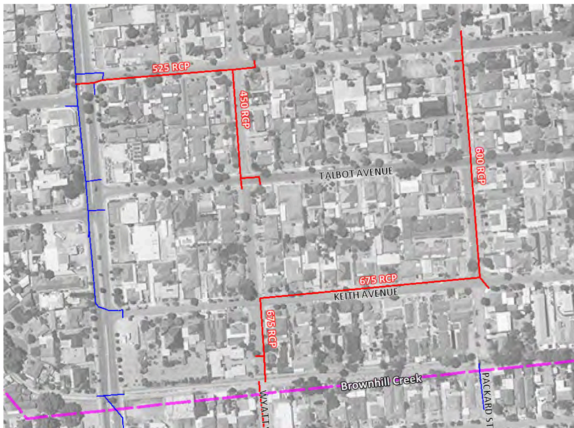
Figure 4.68 – Packard Street Drainage Layout
